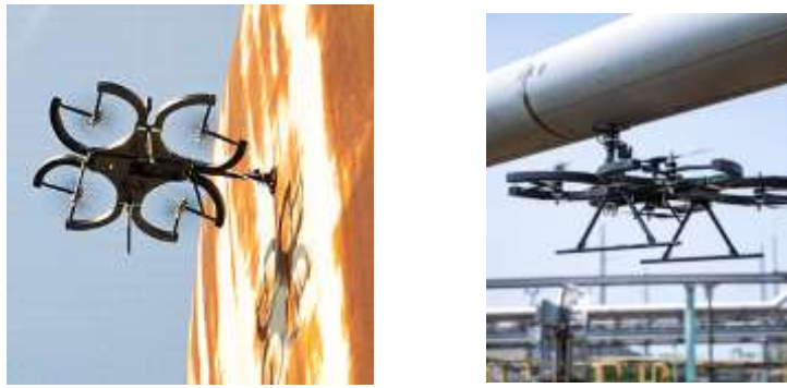
Fig. 1. Drone for Ultrasonic NDT Inspection, designed by Skygauge Robotics
