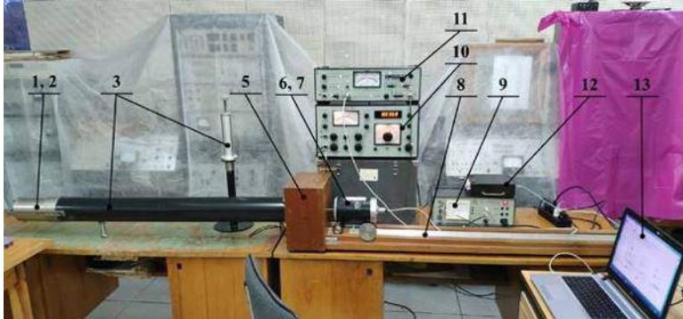
Fig. 1. Experimental apparatus for determining the sound-absorbing characteristics of acoustic liners using the standing wave ratio method
