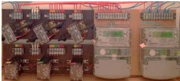
Fig. 1. Laboratory facility for metering unit operation study under reduced load
