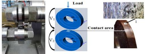
Fig. 2. The diagram of the loading node of the test samples with rotation at speeds  $V_1$  and  $V_2$  and the appearance of the friction tracks of the 30ChGSA steel sample; 1 – section of the contact surface of the sample.
