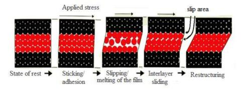
Fig. 1. The influence of shear stress on the lubricating film's deformation and its structure's reorganization [4].
