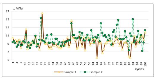
Fig. 3. Kinetics of changes in shear stress of the lubricating layer in contact  $(\tau)$ .
