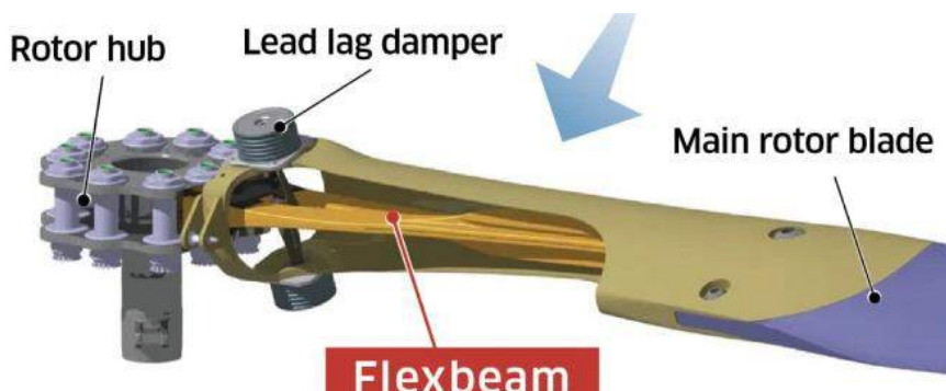
Figure 1. Bearingless rotor system design
